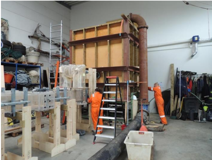
Fig 2a: The 3m Header tank with associated water inlet pipe and connection to the VETT device.
