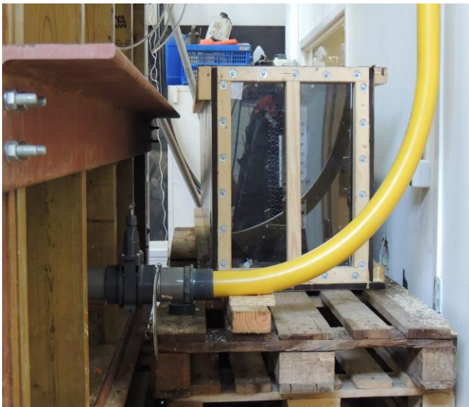
Fig 4a (left): Fish entry mechanism to allow the controlled entry of test fish into the VETT apparatus.
