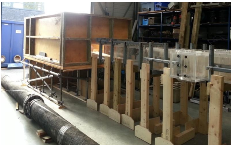
Fig 2b: Sink Tank, showing connection to the Reservoir and the VETT device.
