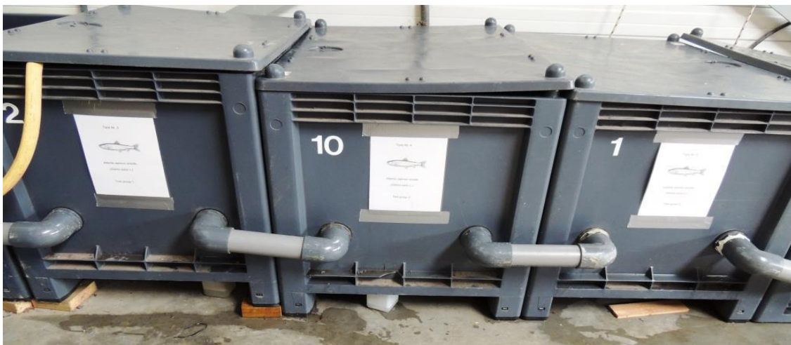
Fig 3b: Test fish storage tanks at VisAdvies, showing the circulation water system which supplied fresh, aerated water to the system during the trial.
