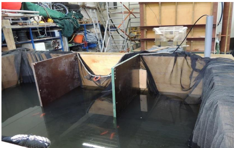
Fig 2c: Sink Tank, showing capture netting and internal baffle structures to provide calm areas for fish to rest in after passage through the VETT.
